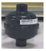
This miniature, completely disposable filter is designed for use with the lightweight, low amperage plasma cutting systems that do not have sufficient space to install one of the larger air filters. Designed for installation in the air hose downstream of the air regulator, the filter has a rated flow of 1,800 SCFH and the ports are 1/4" NPT(F). With the assumption that these small plasma cutting systems are used infrequently, the estimated life of the filter should be several weeks.
