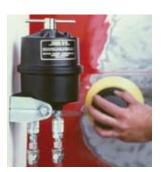
This filter is recommended for use with the larger, stationary plasma cutting systems used for high volume and production cutting on industrial applications. Specifically designed to be mounted in the outlet of the rigid compressed air line adjacent to the plasma system, the filter is equipped with 1/2" NPT ports, and the rated flow is 6,000 SCFH.
