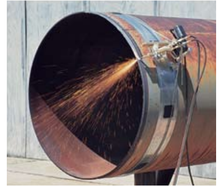
Band Style Cutting 48" Pipe
